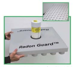
**Radon Guard™** insulation is a patent-pending sub-slab depressurization panel. The interconnected channels on the underside of the panel direct soil gas movement between the ground and the air barrier system to a vent pipe in slab on ground applications as required by National Building Code of Canada 2010, Section 9.13.4. The vent pipe is required to connect to a radon gas mitigation system as per applicable code.
